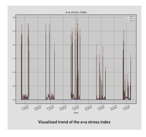
The voltage peak analyser allows the automated measurement, calculation and continuous recording of the e+a stress index over a large period of time without requiring further measurement devices.
